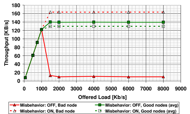
Fig. 10 Throughput vs. offered load for BK vs. Vo priority scenario
