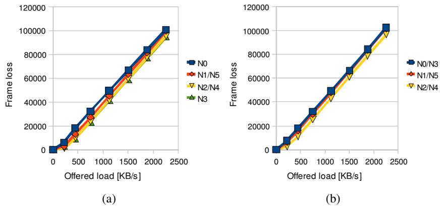
Fig. 5. 6-node ring. Frame loss ( $N_0=P_3$ , others  $=P_0$ ): (a) RTS on (b) RTS off.
