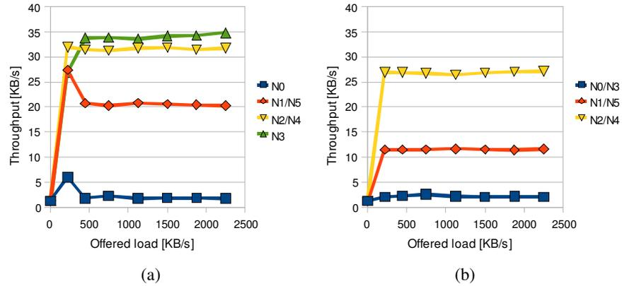
Fig. 4. 6-node ring. Throughput ( $N_0=P_3$ , others  $=P_0$ ): (a) RTS on (b) RTS off.
