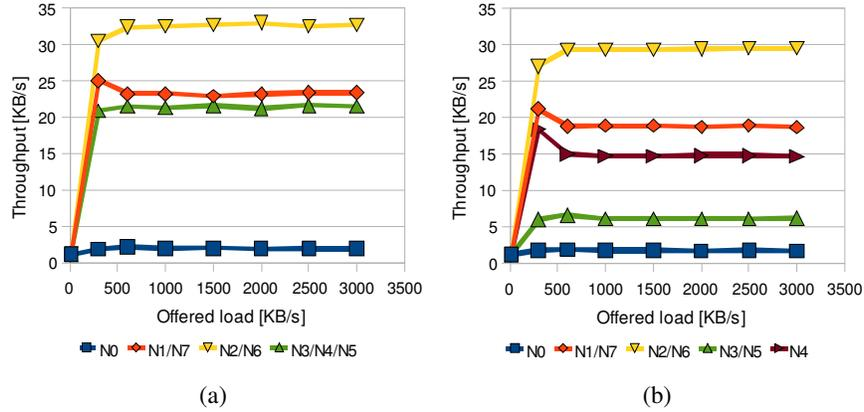
Fig. 7. 8-node ring. Throughput (N0=P3, others =P0): (a) RTS on (b) RTS off.
