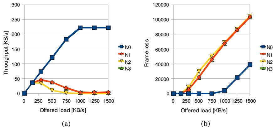
Fig. 3. 4-node ring (N0=P0, others =P3, RTS on): (a) throughput (b) frame loss.
