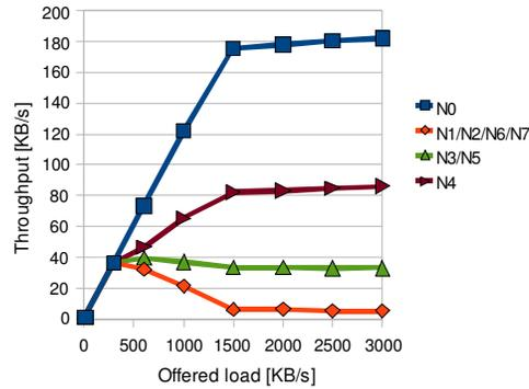
Fig. 8. 8-node ring. Throughput (N0=P0, others =P3): RTS on.
