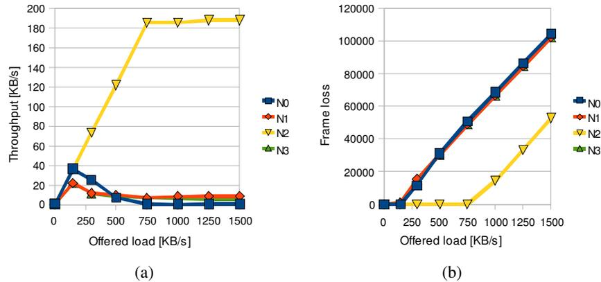
Fig. 2. 4-node ring (N0=P3, others =P0, RTS on): (a) throughput (b) frame loss.
